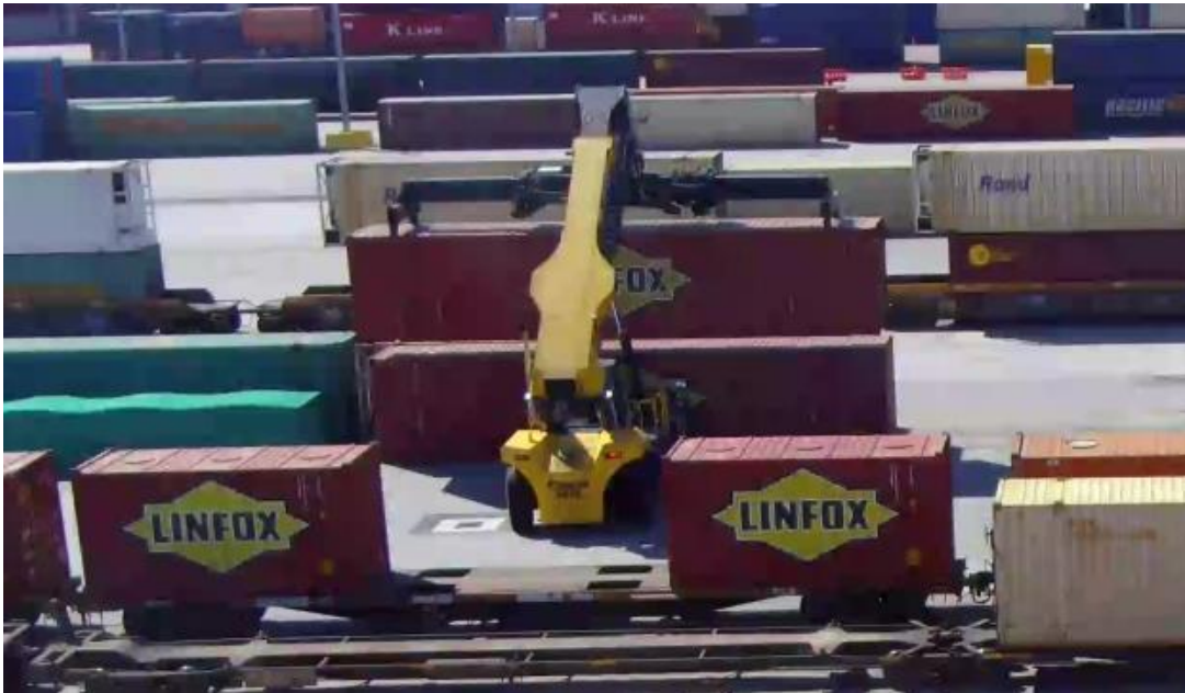
Photo 1: Reach Stacker top lift from container stack
