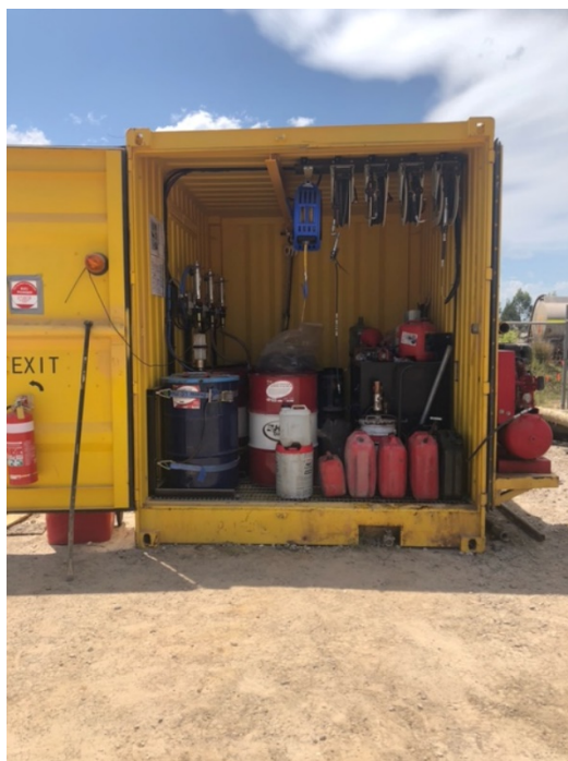
Bunded storage area
