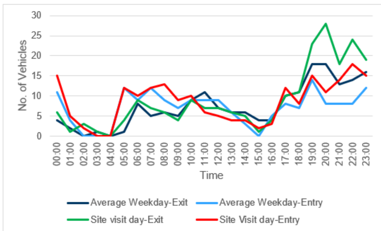
Figure 4.4 Average Weekday and Site Visit profile on the terminal heavy vehicle access road
